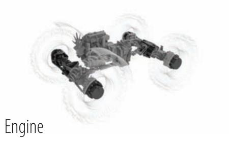
The ALPHA Series engine is one of the most economical and durable in its class. The turbocharged, 4.400 cm<sup>3</sup> engine maintains high torque even at low rpms.
