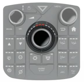
The **TIPSHIFT** function provides operator ease of operation. It is possible to change the direction quickly by pressing a single key without using the gear lever when the machine is moving forward or backward while taking under the load or unloading. This increases productivity and ensures safe operation without the loss of steering control.
