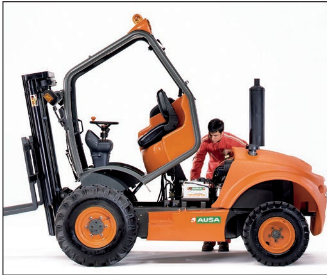
Tilting cab for an easy periodic inspection
